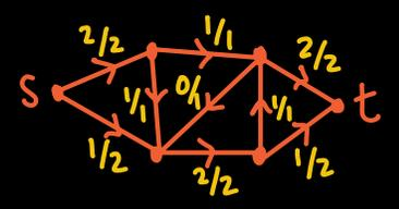
Let  $U = \{u \in V : \exists \text{ a path in } D_f \text{ from } s \text{ to } u\}$
