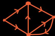
A function  $f: A \rightarrow \mathbb{R}_{\geq 0}$  is called an s-t flow for  $s, t \in V$  if  $\sum_{a \in \mathcal{S}^{\text{in}}(v)} f(a) = \sum_{a \in \mathcal{S}^{\text{out}}(v)} f(a)$  for all  $v \in V \setminus \{s, t\}$
