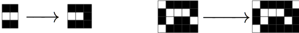
FIGURE 5. Two examples of loops: when a new column is added, the cluster count may decrease, as clusters are connected via the new column.
