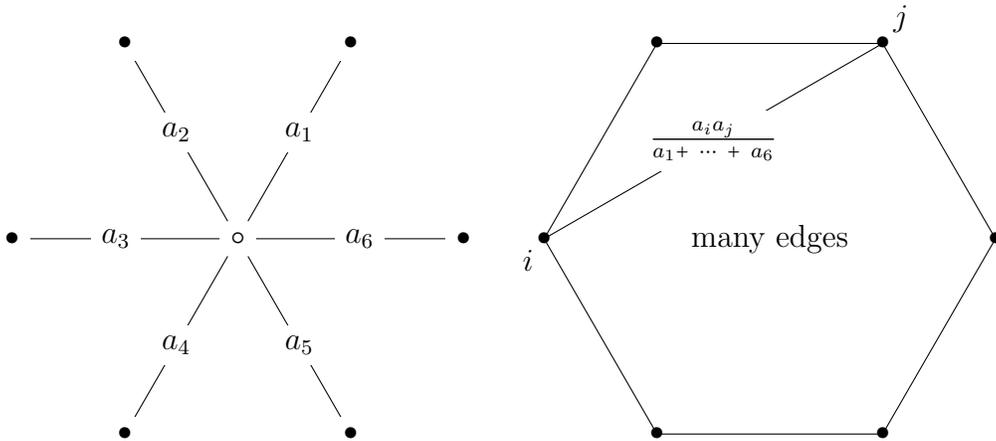
Figure 4: The Star-K transform from a 6-star to a  $K_6$ .
