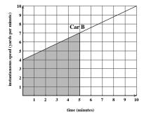
In general, given the graph of instantaneous speed, distance traveled from t = a to t = b is equal to the area of the region under the speed graph and above the t-axis from t = a to t = b.
