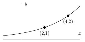
**Solution**. I want a function of either the form  $y = Ce^{kx}$  or the form  $y = Ca^x$ . The curve goes through the points (2, 1) and (4, 2). I'll do both cases.
