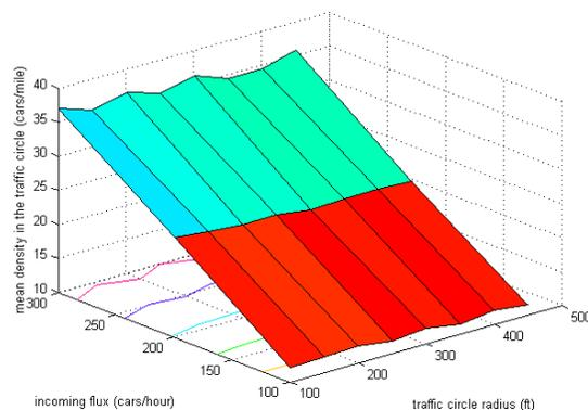
Figure 6: Density for different incoming fluxes and Radii
