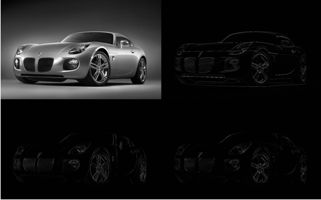
Figure 2: The coefficients of the scale 1 (i.e. j = 1 ) decomposing of the original image. Going clockwise from up-left corner, they are c_1, d_1^v, d_1^h, d_1^d respectively.
