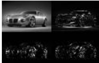
Figure 3: The coefficients of the scale 5 (i.e. j = 5 ) decomposing of the original image. Going clockwise from up-left corner, they are c_5, d_5^v, d_5^h, d_5^d respectively.
