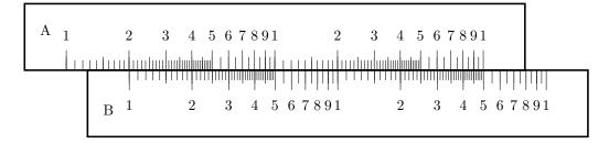
3. Find the 3 on scale B, and see where it lines up to on scale A. This is the answer!
