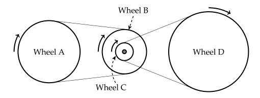
Suppose Wheel A has radius 8 cm, Wheel B has radius 5 cm, Wheel C has radius 2 cm, and Wheel D has radius 9 cm.
