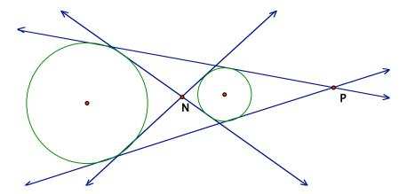
The point P is the center of a dilation that takes one of the circles to the other with a positive dilation ratio equal to a ratio of the radii. The point N is the center of a dilation that has a negative dilation ratio. Once the points P and N are constructed, it is only necessary to construct the tangents from the point to one of the circles and the tangent lines will also be tangent to the other circle. (There is some reasoning required to justify this statement.)
