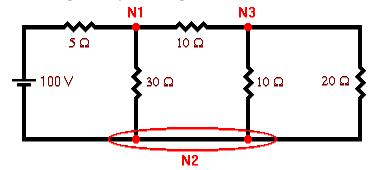
N2 is the reference node as so the voltage is 0V.
