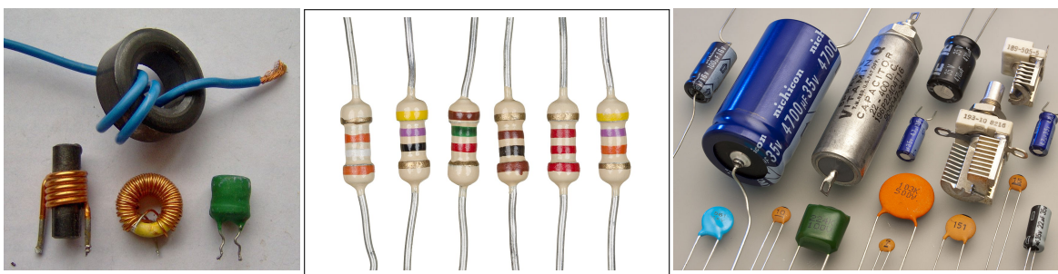
FIGURE 1.3. An assortment of inductors (left), resistors (center), and capacitors (right). (Photograph of inductors by F. Dominec. Photograph of capacitors by Eric Schrader.)
