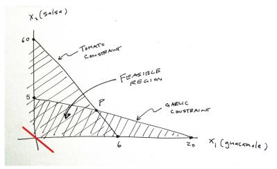
Since the level curves have slope -1, and -10 < -1 < -0.25, we can conclude that the level curves will last hit the feasible region at P, the intersection of the two constraint lines.
