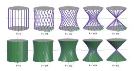
Ruling Lines and Fun Facts: A ruling line is a line that is completely contained on a surface in 3D. A hyperboloid is unusual because it is a curved surface on which every point on the surface is on a ruling line. Another fun fact is that if you take two circular parallel rings, attach elastic string vertically between them, and slowly rotate the bottom, then all the lines formed by the strings will be on the same hyperboloid. Visuals at various angles of rotation,  $\theta$ , are shown above.
