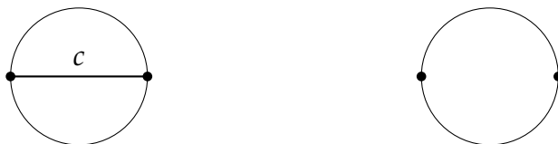
Figure 1: The electrical networks with response matrix L = \begin{bmatrix} -c & c \\ c & -c \end{bmatrix} for c > 0 and c = 0 .
