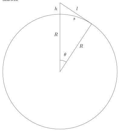
Here h is our height (or the height of our eye) above sea level, R is the radius of the earth, l is the length of the line connecting our eye directly to the horizon, and s is the arc length, the distance along the surface of the earth to the horizon. The angle  $\theta$  is the angle made between our position and the horizon.
