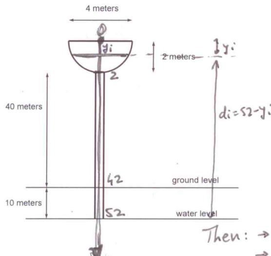
Since we have to compute this integral, it's best to set up the coordinate system with origin at the top (center of circle) and positive direction downwards
