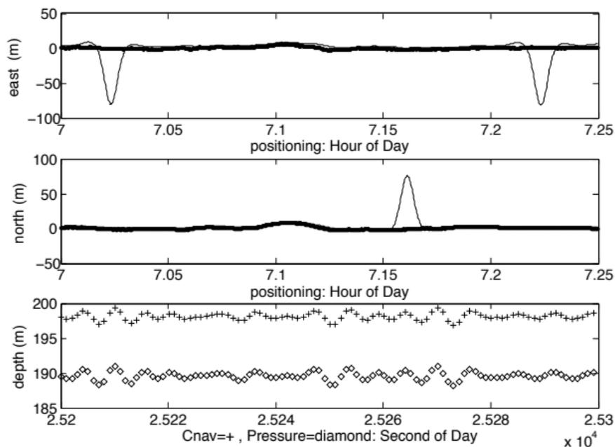
Figure : Track: Independent GPS verification (thick line and +), Iterated Gaussian smoother estimate (thin line).
