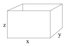
Label the sides as shown. The cost is C = 3xy + 4xz + 4yz. The volume constraint is xyz = 6.
