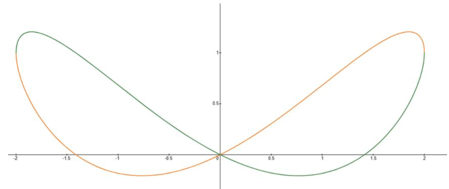
This is what the side view of the intersection of a cylinder and sphere looks like.
